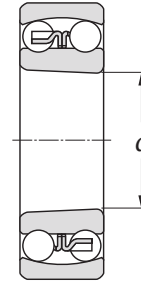
Tapered bore taper 1:12
