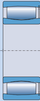
Full complement bearing For very heavy loads and low speeds
