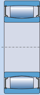
Sealed bearing Lubricated for life and protected against contaminants, for heavy loads and low speeds
